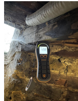
Photo 182 - Stained timber generally dry when tested
