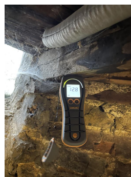
Photo 187 - Stained timber generally dry when tested
