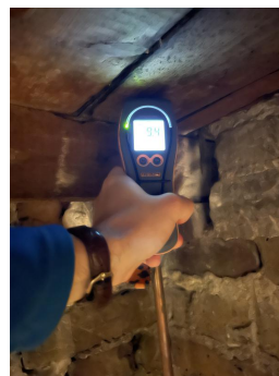
Photo 185 - Stained timber generally dry when tested
